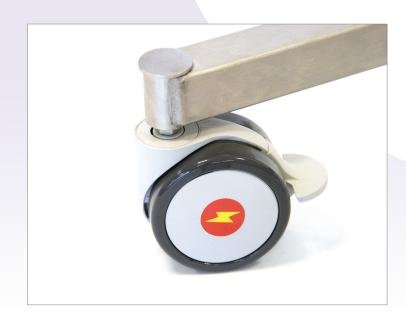
Another significant improvement in the RMA IV pole design is the use of solid machined bushes for castors fixing eliminating the need for threaded inserts that can become loose and unserviceable over time. The new RMA IV Pole is also fitted with two anti-static rust resistant 75mm castors.
