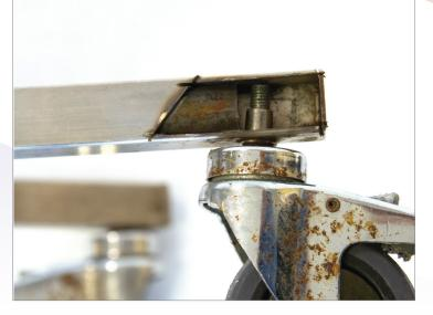
Above: Example of damaged, inferior threaded inserts and rust tarnished castor forks.
